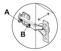
1) **Side to side adjustment:** Loosen screw **A**, adjust gap with screw **B** and re-tighten
